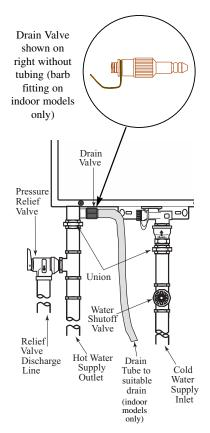
**Notice**: The above illustrates a pressure-only relief valve. If local codes require a combination temperature and pressure relief valve be installed, an extension piece may be needed to ensure that the valve probe is not directly in the flow path of the water.
